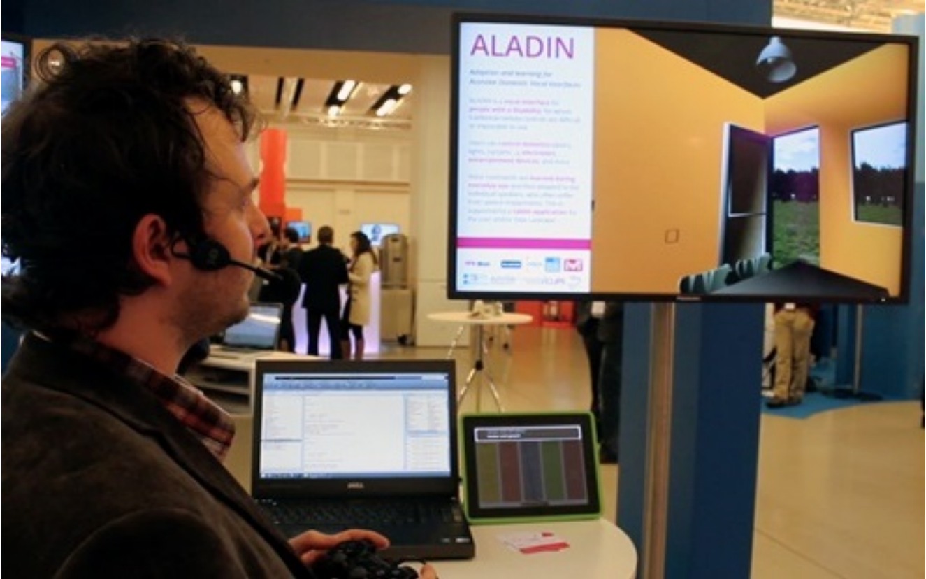
Figure 3: Demo setup. In the top-right corner, the interactive 3D home environment is shown. The VUI is running on the laptop, with the companion tablet shown to the right. The demo staff operating the VUI is using a wireless microphone and a game controller. A far-field microphone and actual home automation setup are also supported (not shown).
