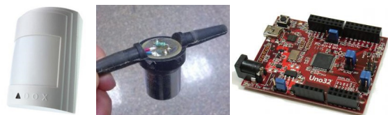
Figure 1. Images of the PIR sensor, the vibration sensor, and the Uno32 microprocessor, from left to right, respectively.
